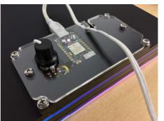
Ensure solder connections are sound, with no bridging. Rotate pot to far-left. Plug power supply into Photon - LED should glow white. Slowly
