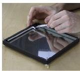
Line the mirror-box walls with double-sided adhesive tape and press the LED strip into position: Position soldered-end of strip so wires exit upwards through corner cutout. Make sure the strip follows the rounded corners closely. The ends of the strip should not contact eachother.
