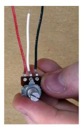
• Cut 70mm of each Red and Black wire, 40mm of White. Strip 5mm of insulation from each end. • Solder as shown and remove the mounting nut and washer from the pot -
