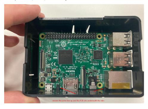
Press gently on the top of the board to snap the locking lug into place.
