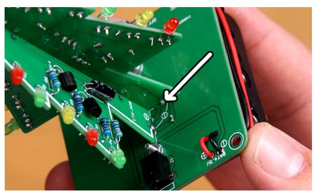
Where PCB A and B meet there are a series of solder pads that can be joined to better hold the 2 PCBs together.
