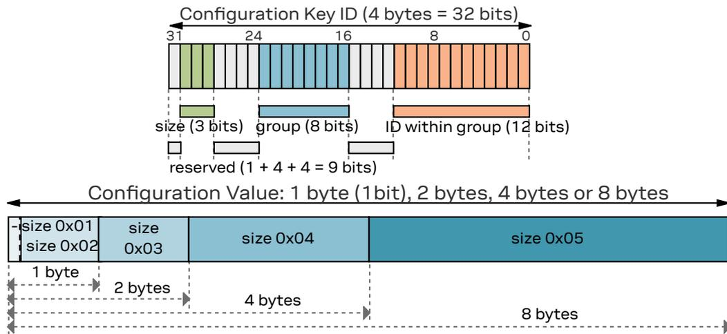
A Configuration Key ID is a 32-bit integer value, which is split into the following parts:
