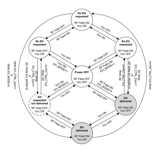
Note: Power is delivered on V\_EH only if harvested energy is sufficient to supply ST25DVxxKC and leave over power.
