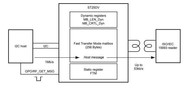
Figure 11. I<sup>2</sup>C to RF fast transfer mode operation
