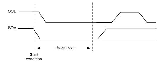
Figure 30. I<sup>2</sup>C timeout on Start condition
