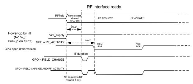
Figure 7. ST25DVxxKC RF power-up sequence (No DC supply)
