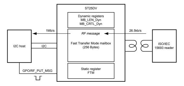
Figure 10. RF to I<sup>2</sup>C fast transfer mode operation
