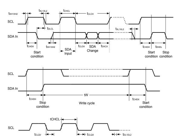
Figure 80. I<sup>2</sup>C AC waveforms
