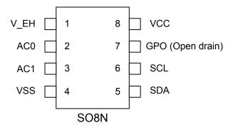
Figure 3. ST25DVxxKC 8-pin TSSOP8 package connections
