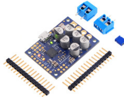
High-Power Simple Motor Controller G2 24v19 with included hardware.
