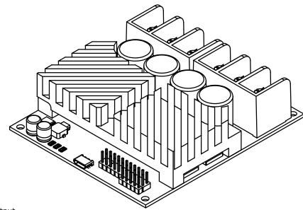
The RoboClaw is an intelligent, high performance motor controller designed to control dual brushed DC motors. It can be controlled from USB, RC radio, PWM, TTL serial, analog and microcontrollers such as an Arduino or Raspberry Pi.
