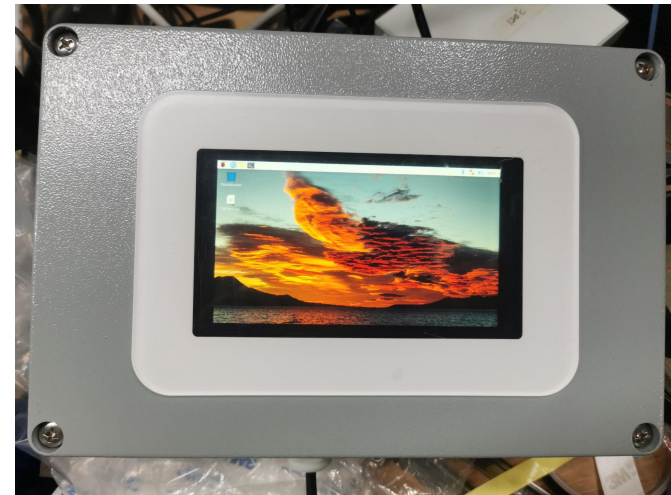
SCADA HMI, Panel PC
