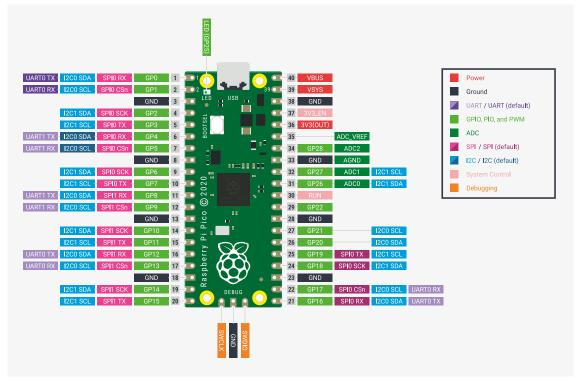
Pico uses an on-board buck-boost SMPS which is able to generate the required 3.3 volts (to power RP2040 and external circuitry) from a wide range of input voltages (~1.8 to 5.5V). This allows significant flexibility in powering the unit from various sources such as a single Lithium-Ion cell, or 3 AA cells in series. Battery chargers can also be very easily integrated with the Pico powerchain.
