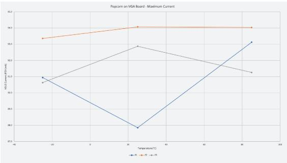
Table 2. Popcorn running on the VGA Board (VGA video, SD Card and I2S audio) with power saving disabled (GPI023 pulled high)
