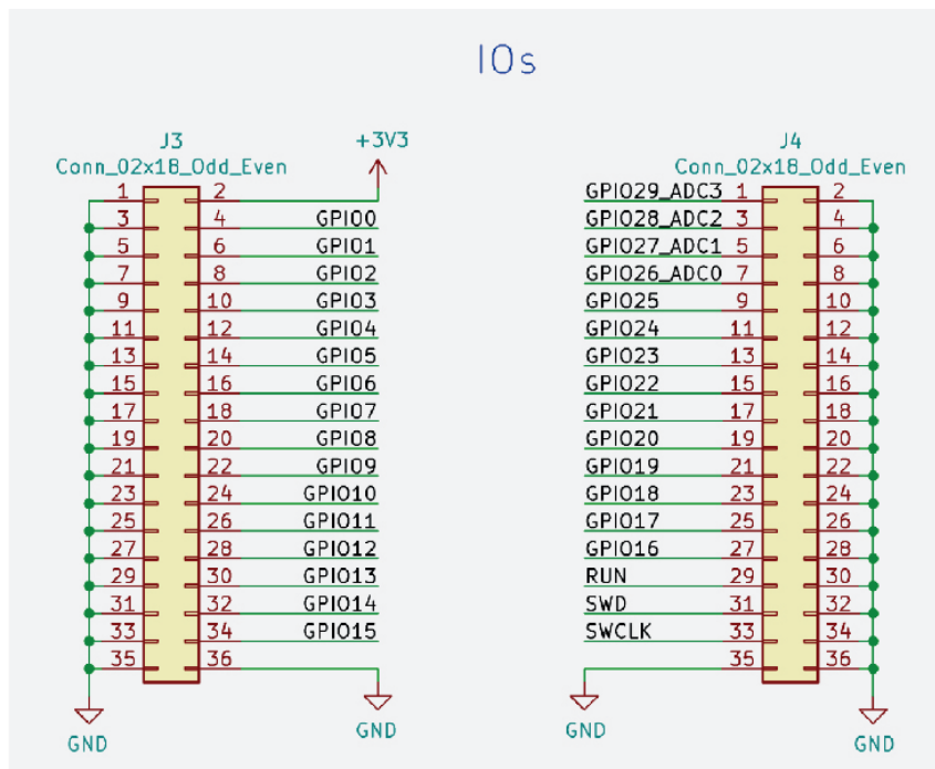
Figure 10. Schematic section showing the 2.54mm IO headers
