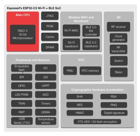
Figure 1: Block Diagram of ESP32-C3
