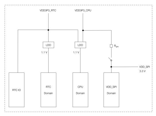
Figure 4: ESP32-C3 Family Power Scheme
