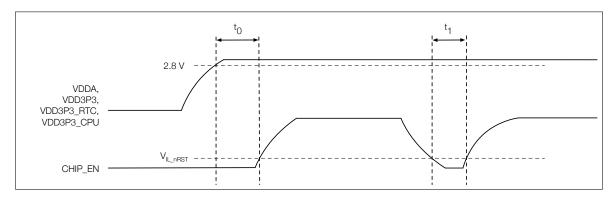
Figure 5: ESP32-C3 Family Power-up and Reset Timing
