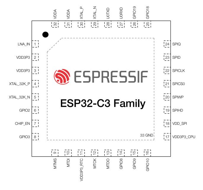
Figure 3: ESP32-C3 Pin Layout (Top View)
