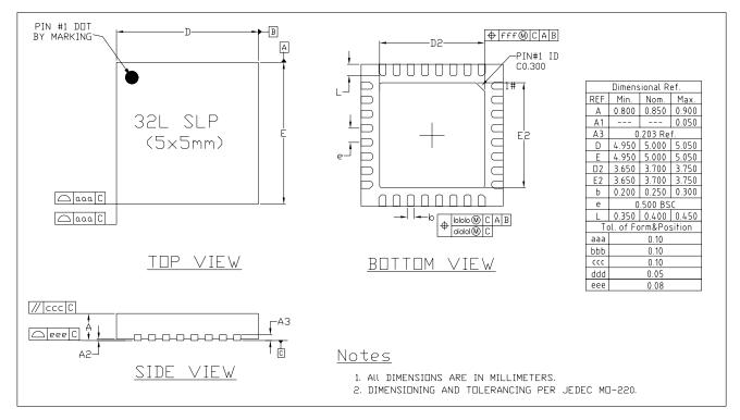
Figure 8: QFN32 (5×5 mm) Package
