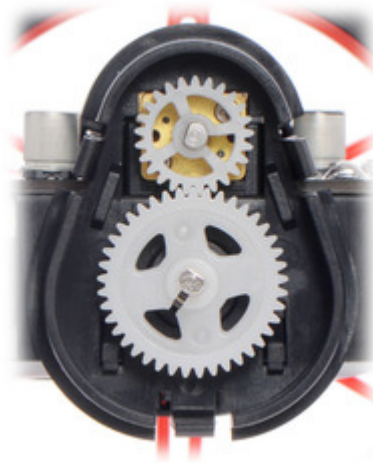
A look inside the external gearbox on the Balboa 32U4 Balancing Robot.
