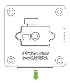
2. Insert the ribbon cable with pins facing away from the catch.
