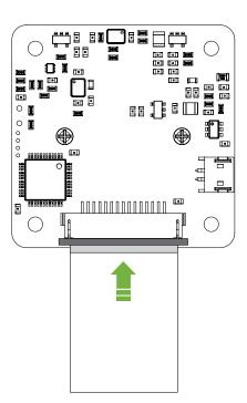
4. Connect the camera to Jetson Nano/NX, with pins facing away from the catch.
