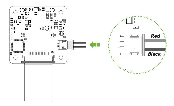
6. Connect the 2-pin cable to Jetson Nano's GPIO (5V & GND)
