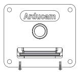
2. Insert the ribbon cable with pins facing away from the catch.
