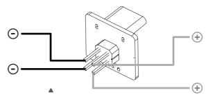
12. Polarity diagram of fan adapter.
