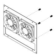
1. Install the fan to the back panel. Pay attention to the direction of the fan, the stickers should face the Raspberry Pi.
