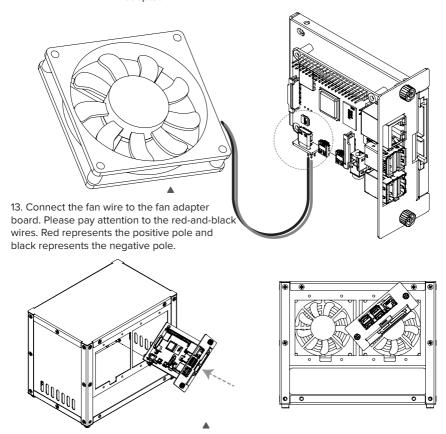
14. Tilt and insert the installed bracket into the case and fix it with Captive Loose-Off Screws.
