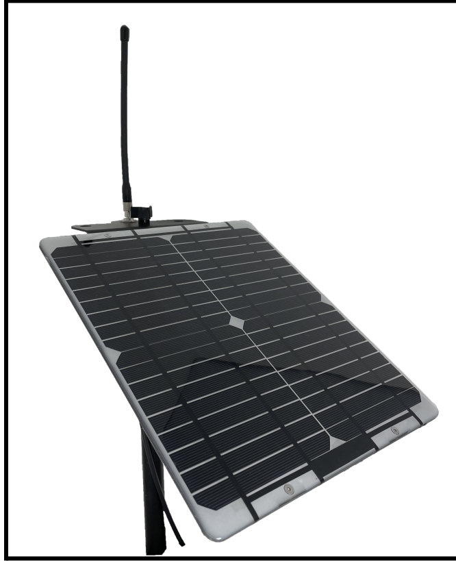
Figure 10: Example \frac{1}{4} -wave antenna with a (Swarm) 9W solar panel serving as the required 30 x 30 cm ground plane off to one side. Tested extensively in the field and works well.
