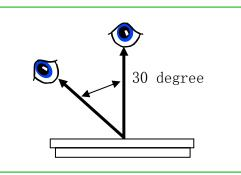
Under daylight lamp 20 $\sim40W_{\textrm{P}}$  product distance inspector'eye 30cm,incline degree 30°.
