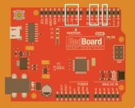
off so that it is only on 50 percent of the time (50% of 5V is 2.5V). By doing this, any voltage between 0 and 5V can be produced. This is what is known as Pulse-Width Modulation (PWM). It can create many different colors on the RGB LED.
