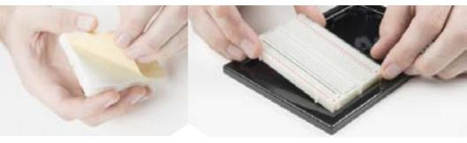
**PEEL** the adhesive backing off the breadboard.
