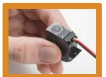
**ATTACHING YOUR SERVO:** A strip of adhesive Dual Lock<sup>™</sup> fastening tape is included in your kit. Cut two pieces of it to temporarily affix your servo to your baseplate.
