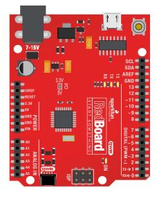
**THE SPARKFUN REDBOARD QWIIC** is one of a multitude of development boards based on the ATmega328 microprocessor. It has 14 digital input/output pins (six of which can be PWM outputs), six analog inputs, a 16MHz crystal oscillator, a USB connection, a power jack, and a reset button. You'll learn more about each of the RedBoard's features as you progress through this guide.
