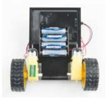
so that the two pieces of Dual Lock snap together. Insert the batteries into the holder if you have not done so already. Remember that batteries are polarized and can only go in one way.
