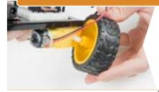
**5. ATTACH THE WHEELS** by sliding them onto the plastic shafts on the gearmotor. The shaft is flat on one side, as is the wheel coupler. Align the two, and then press to fit the wheel onto the shaft.
