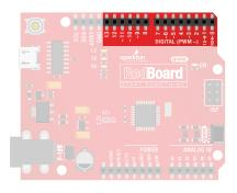
**DIGITAL OUTPUT:** When working with microcontrollers such as the RedBoard, there are a variety of pins to which you can connect electronic components. Knowing which pins perform which functions is important when building your circuit. In this circuit, we will be using what is known as a digital output. There are 14 of these pins found on the RedBoard. A digital output only has **two states: ON or OFF.** These two states can also be thought of
