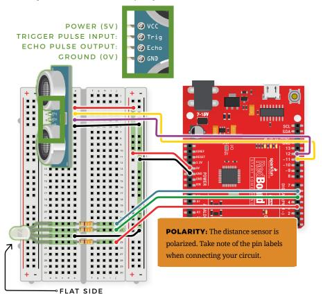
CONNECTION TYPES REDBOARD CONNECTION = BREADBOARD CONNECTION
