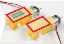
**3. PRESS THE MOTORS TO THE BASEPLATE,** connecting the two Dual Lock surfaces. Try to get the motors as straight as possible so your robot will drive straight.
