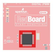
INTEGRATED CIRCUITS (ICS) AND BREAKOUT BOARDS: An Integrated Circuit (IC) is a collection of electronic components — resistors, transistors, capacitors, etc. — all stuffed into a tiny chip and connected together to achieve a common goal. They come in all sorts of flavors, shapes and sizes. The chip that powers the RedBoard, the ATmega328, is an IC. The chip on the motor driver, the TB6612FNG, is another IC.
