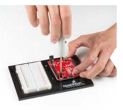
ALIGN THE REDBOARD with its spot on the baseplate. The text on it should face the same direction as the text on the breadboard and the baseplate. Using one of the two included screws, affix the RedBoard to one of the four stand-off holes found on the baseplate. The plastic holes are not threaded, so you will need to apply pressure as you twist the screwdriver.
