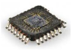
The guts of an integrated circuit, visible after removing the top.
