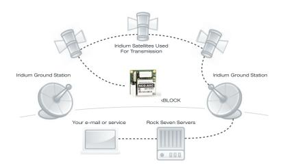
The RockBLOCK allows you to send and receive short messages from anywhere on Earth with a clear view of the sky. It works far beyond the reach of WiFi and GSM networks.
