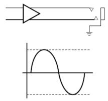
The TrueCapFree amplifiers require no output DC-blocking capacitors. The headphone connector shield pin connects to ground and will interface with headphones and non-headphone accessories. The PAM8908 is an amplifier.
