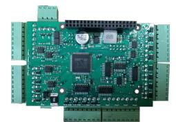
The second generation of our Industrial Automation card brings to the Raspberry Pi platform all the building blocks required for Industrial Automation projects. Stackable to 8 levels, the card works with all Raspberry Pi versions, from Zero to 4.
