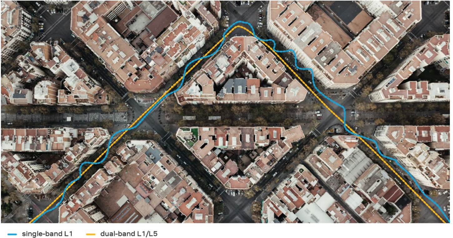
Figure 6. Car drive test in an urban environment comparing L1 vs. L1/L5 band GNSS
