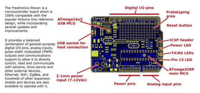
All I/O pins and power rails are brought out to convenient headers, allowing you to either connect individual pins to a breadboard using standard jumper wires or to plug in "shield" daughter-boards for versatile expansion. General-purpose prototyping shields are also available which provide extensive space for you to create your own add-on circuits.
