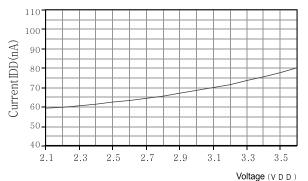
Figure 7 shows the typical relationship between supply current and voltage (dormancy mode) at 25  $^\circ$ C. Please be noted that the deviation between these data and the display value may reach  $\pm$  50 % of the display value. At 60  $^\circ$ C, the coefficient is about 15. (Compared with Table 2).
