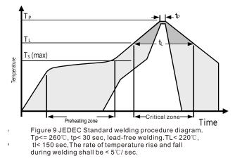
AHT 20 can be welded through standard reflow furnace. The sensor fully meets the IPC/JEDEC J-STD-020D welding standard. The contact time should be less than 30 seconds at the highest  $260^{\circ}$  (see Fig. 9) and the ultimate welding temperature that the sensor can withstand is  $260^{\circ}$ , so it is recommended to use low temperature  $180^{\circ}$ when reflow soldering.
