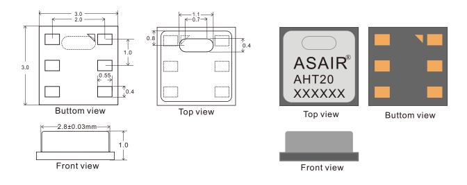
Figure 1: AHT20 Sensor Package Diagram (Unit: mm Tolerance: 0.1 mm)
