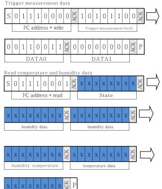
Note: The sensor takes time to collect data. After the host sends out the measurement command (0 x AC), it delays more than 75 milliseconds to read the converted data and judge whether the returned status bits are normal. If the state bit [Bit 7] is 0, the data can be read normally, and 1 represents that the sensor is busy, the host needs to wait for data processing to complete.
