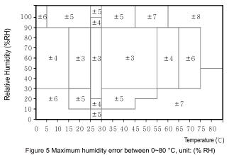
Note: Above errors are the tested maximum errors (excluding hysteresis) with the high precision dew-point instrument as reference instrument. The typical error is  $\pm 2$  % RH with the range of maximum error. In other scopes, the typical value is 1/2 of the maximum error.
