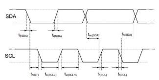
Figure 12.The sequence diagrams and abbreviations of digital input/output are explained in Table 8. Thicker SDA lines are controlled by sensors, and ordinary SDA lines are controlled by single chip computer. Please be noted that the effective read time of SDA is triggered by the drop edge of the previous conversion
