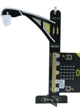
**Connection:** 4 x M3 countersunk screws allow the user to bolt the LAMP:bit onto the BBC micro:bit.
