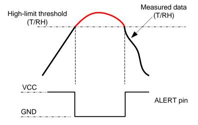
Figure 10. ALERT pin logic status
