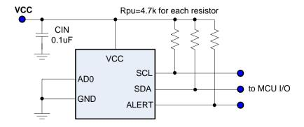
Figure 1. Typical Application of CHT8305C
