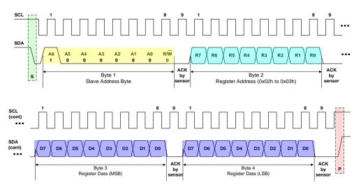
Figure 8. I<sup>2</sup>C Write Word (2-Bytes) Timing Diagram
