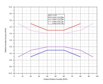
Figure 4. Relative Humidity Accuracy
