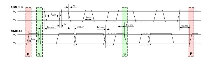
Figure 7. I<sup>2</sup>C Timing Diagram
