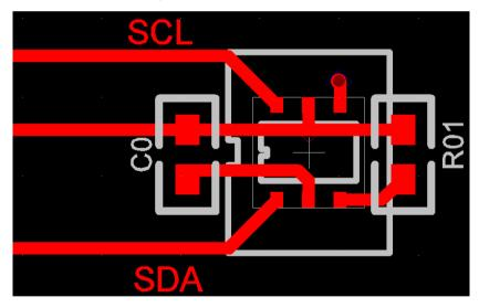
Figure 13. Sensor PCB layout example
