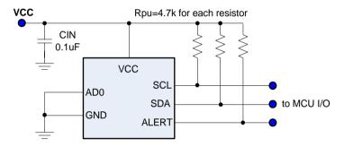
Figure 11. Sensor typical application
