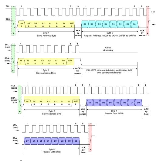
Figure 9. I<sup>2</sup>C Read Word (2-Bytes, for temperature or humidity) Timing Diagram
