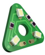
NOTE: Care should be taken when soldering to the + and – pads so that the surface mount LEDs are not inadvertently damaged
