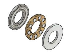
**Pro Tip:** Thrust bearings have two thrust washers and a ball carriage which go together as shown here, with the grooves towards the balls.
