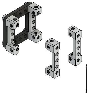
Using eight 9mm length M4 screws, attach the dual block mounts to the slide plates. Note the orientation of the dual block mounts.
