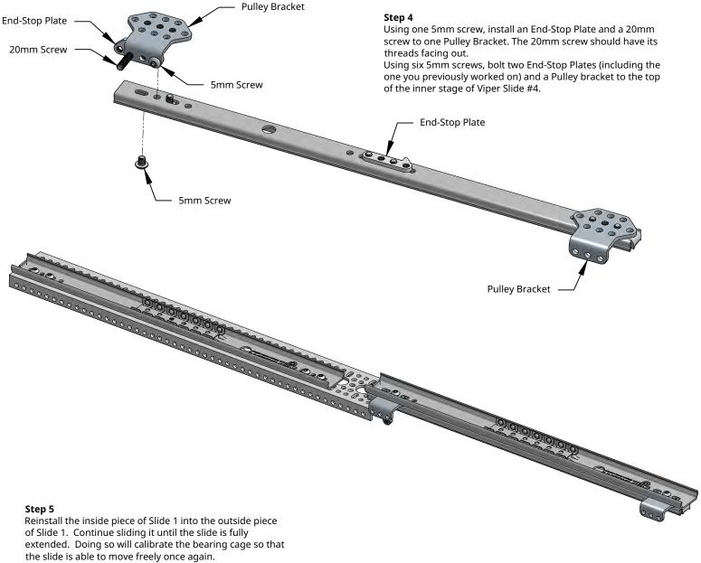
Repeat this process twice, adding a stage of assembles you made in step 3 with each, as shown below.
