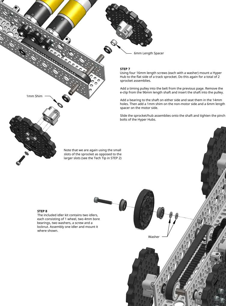
You now have one "track pod" minus the track segments. Repeat Steps 1-8 to create the other track pod for this chassis. Note that the second track pod needs to be a mirror image of the first.
