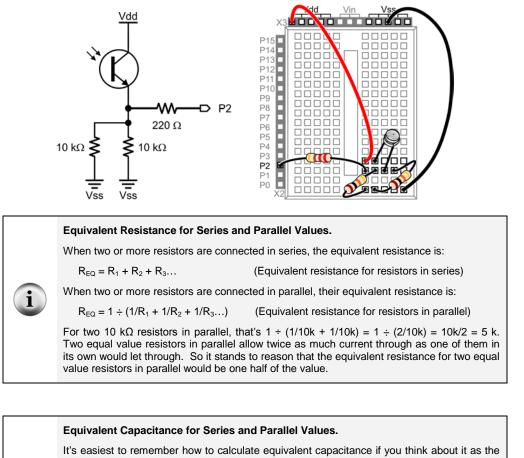
It's easiest to remember how to calculate equivalent capacitance if you think about it as the reverse of series and parallel resistor calculations. So, the equivalent capacitance for parallel capacitors adds up, and equivalent capacitance for series capacitors uses inverses.
