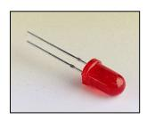
An LED is a special diode. LED stands for Light Emitting Diode. LEDs are like normal diodes, in that they only allow current to flow in one direction, however, when the current is flowing, the LED lights up.
