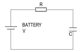
When a capacitor is connected to an item such as a battery, or in this kit a solar cell, charge will flow from the battery into it. Therefore, the capacitor will begin to fill up. The flow of water in the picture above left is the equivalent of how the electrical charge will flow in the circuit shown on the right.
