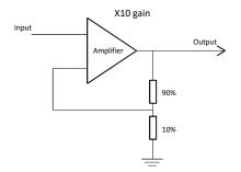
With an infinite gain the amplifier is no good to amplify audio, which is where the feedback comes in. By making one of the inputs a percentage of the output the gain can be fixed, which allows the output to be a copy of the input but bigger. Now when the two inputs are compared and the output is adjusted, instead of it going up or down until it reaches 0 volts or V+, it stops at the point when the two inputs match and the output is at the required voltage.
