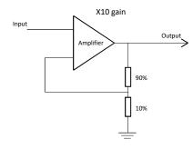
With an infinite gain the amplifier is no good to amplify audio, which is where the feedback comes in. By making one of the inputs a percentage of the output the gain can be fixed, which allows the output to be a copy of the input but bigger. Now when the two inputs are compared and the output is adjusted, instead of it going up or down until it reaches 0 volts or V+, it stops at the point when the two inputs match and the output is at the required voltage.
