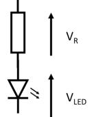
The next nearest preferred value is  $22\Omega$ , which results in an actual current of 21.5 mA per LED, which is in the right range (20-25mA).
