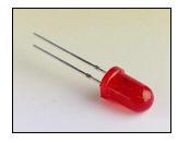
An LED is a special diode. LED stands for Light Emitting Diode. LEDs are like normal diodes, in that they only allow current to flow in one direction, however when the current is flowing the LED lights.
