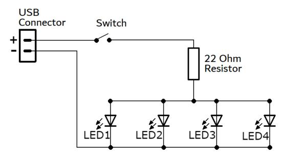
The circuit diagram for the 5V LED Desk Lamp is shown above. It is a very simple circuit. The board contains four LEDs, sharing a current limit resistor.
