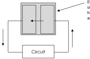
Electrons jump between two silicon layers when the sunlight hits the cell. They then flow around the electric circuit.
