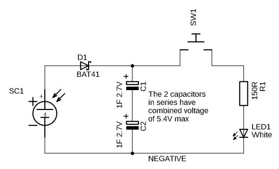
The circuit has 2 distinct sections, an energy storage section – consisting of the capacitors, diode and solar cell, and an energy using section – the LED. The sections are joined by the switch.
