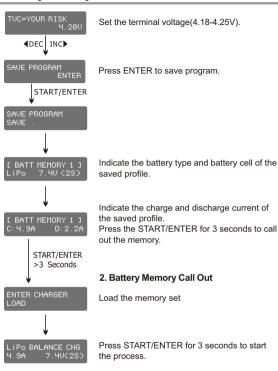
It will be operated with the default value of the essential user settings when it is powered on for the first time. The screen displays the following information in sequence and the user can change the value of parameter on each screen.
