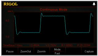
The electronic load provides the waveform display function and supports the following operations for the waveform, such as pausing the waveform, enlarging and narrowing the waveform, and capturing the waveform. Therefore, you can dynamically observe the trend of parameters changes.
