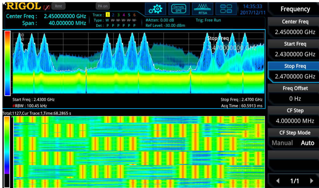
Figure 12: Bluetooth signal measured with density spectrogram
