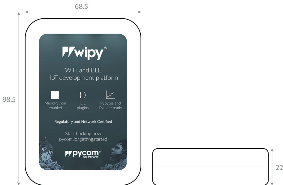
Figure 10 – Mechanical drawing of packaging – Units: mm
